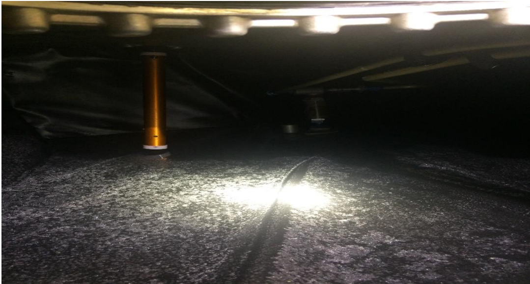
Figure 2: DEF crystallization in aircraft fuel tank.
