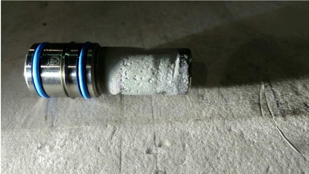
Figure 1: DEF crystallization on aircraft fuel filter.
